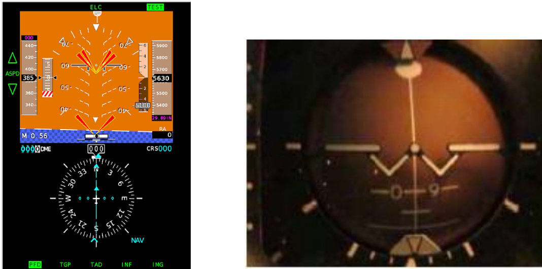
Figure 11: PFD and Standby ADI in Steep Dive with INS INFLT ALIGN (Tabs T-15 and T-20)
